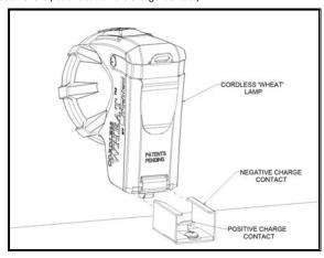
**3.)** Once connected to the charger, the LED status indicator inside the reflector will glow solid red to show that it is charging correctly. Upon completion of the charge cycle, this LED indicator will glow green. At that time, the light is ready to use. However, it can be left on the charger indefinitely without damage to the unit.
