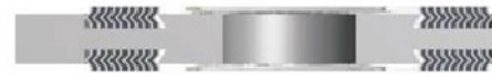
Spiral wound sealing element Machined Carring Gasket Cross-section through Carring Gasket assembly
